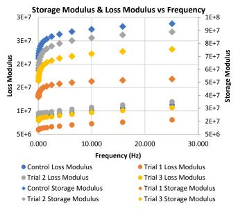
Trial 1 had the highest tan delta at all tested frequencies. This is despite having the lowest loss modulus of all the trials. The higher tan delta figure for Trial 1 is due to the loss in G'.
